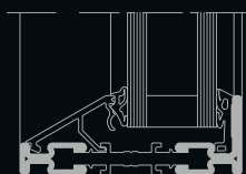
Glasleiste Schräg Inclined glazing bead
