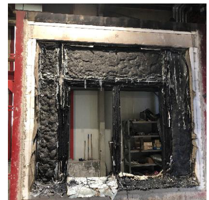
The test is ended after integrity is lost and flames pass through. The fire exposed side can be seen to be charred and molten.
